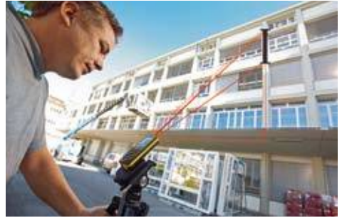
Indirect height-measurement: Window heights can be determined using the Pythagoras function.
